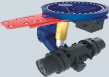
+ Goldhofer driven pendular axle with ball bearing race ring
