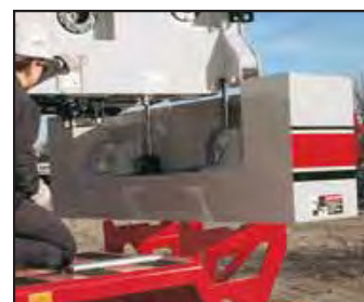
Fast & efficient hydraulic counterweight removal enhances roadability
