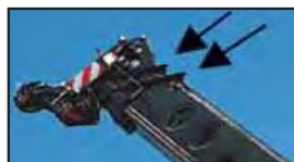
A-max extends only the inner-mid section of the boom for substantially increased capacities for in-close, maximum capacity lifts.
