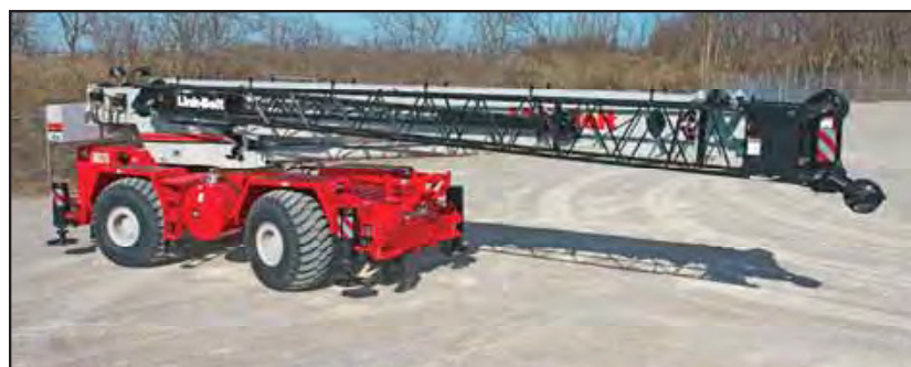
A-max extends only the inner-mid section of the boom for substantially increased capacities for in-close, maximum capacity lifts.
